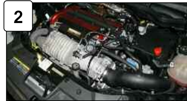
Complete Stock intake. Please disconnect battery terminals before installation. Note: For additional information of air box removal, consult owners manual.
