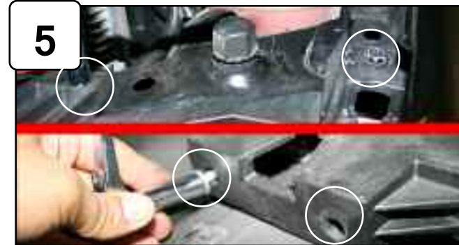
With 10mm socket or wrench, loosen the 4 bolts holding in headlight assembly bracket.
