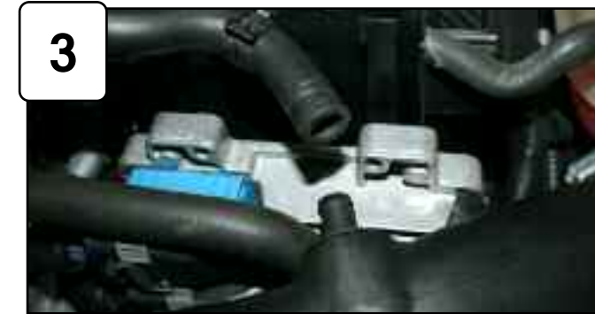
With pliers, pull back crank case line from intake. Loosen clamps using 5/16" nut driver and remove stock upper intake tube.
