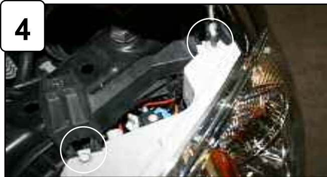
With 10mm socket, remove the 2 bolts holding in the headlight. Carefully pull back and remove headlight. Disconnect harness.
