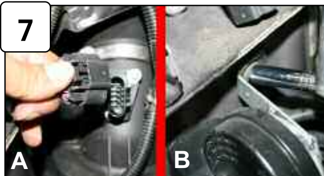
A)Disconnect MAF sensor harness. B)With 10mm socket or wrench, loosen the bolt holding horn bracket and set aside.
