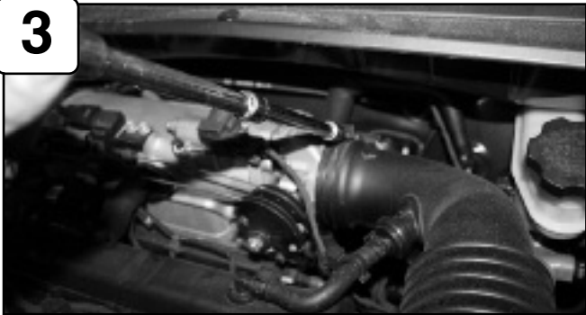
With 10mm socket or wrench, loosen clamp on throttle body.
