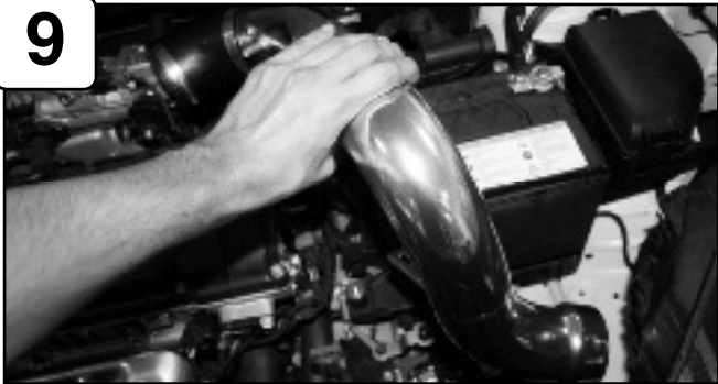
Install upper intake tube assembly into vehicle with provided elbow coupling and clamps. Do not tighten.
