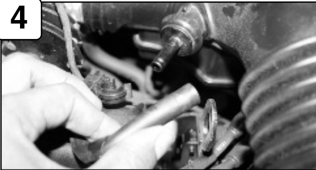
With pliers, remove crank case line from OE intake tube.
