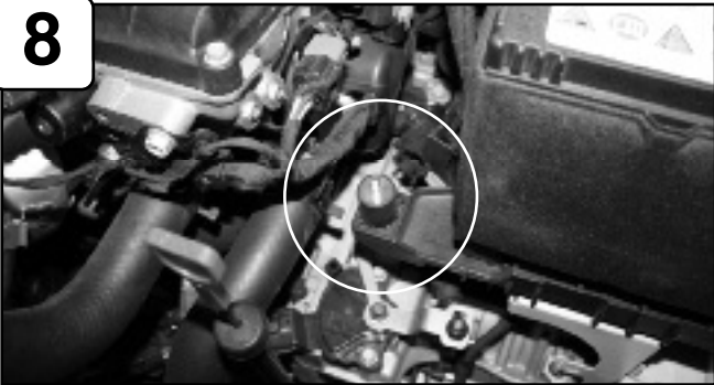
Install provided M6 isolation mount to factory air box mounting point next to battery tray.
