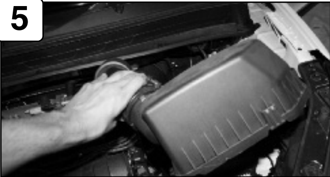
Un-clip upper half of air box and remove.
