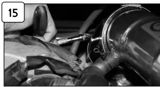
Tighten all remaining clamps using 5/16" nut driver.
