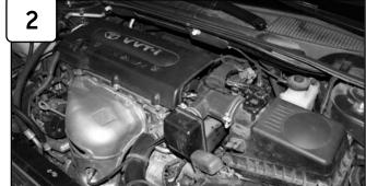
Complete Stock intake. Please disconnect battery terminals before installation. Note: For easier installation engine cover removal is optional.
