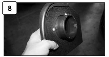
Attach filter adaptor to inside of housing and secure using the 3 button head screws provided. Tighten using 4mm allen key.
