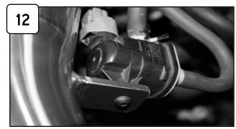
Attach VSV module to bracket on tube and secure using bolt from step 3.
