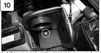
Install housing and position bracket to reservoir from previous step. Secure tab and tighten. With provided hex screw and washer, tighten and secure bottom of housing.
