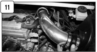
Install tube and position to throttle body and adaptor. Do not tighten.
