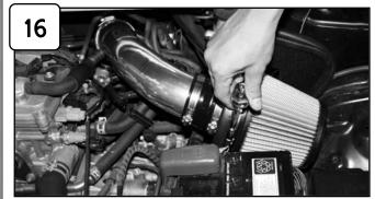
Install filter and tighten using 5/16" nut driver.
