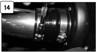
Tighten clamps on adaptor side using 5/16" nut driver.
