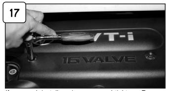
If removed, install engine cover and tighten. Re-connect battery terminals.
