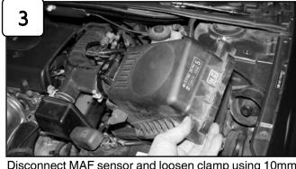
Disconnect MAF sensor and loosen clamp using 10mm socket or wrench. Unclip upper half of air box and remove. With phillips screwdriver loosen VSV module from tube. *Note: Save screw for later install.* Loosen clamp with pliers on throttle body and remove stock intake tube assembly.
