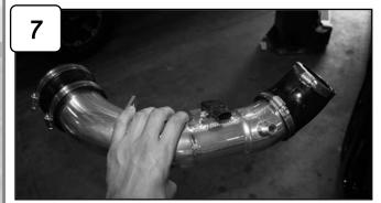
Attach couplings to tube with clamps provided, do not tighten.
