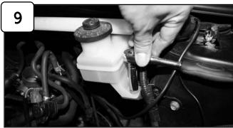
Loosen the screw holding in Fluid reservoir using 10mm socket or wrench and save screw for later install.
