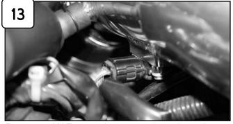
Reconnect MAF sensor harness and attach crank case line to tube.
