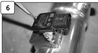
Install MAF sensor into new tube with provided M4 screws and tighten.
