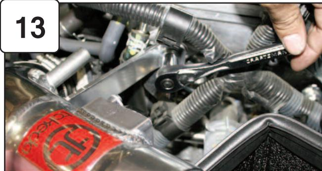
Secure tab on tube to engine. Re-install bolt from step 11 and tighten.
