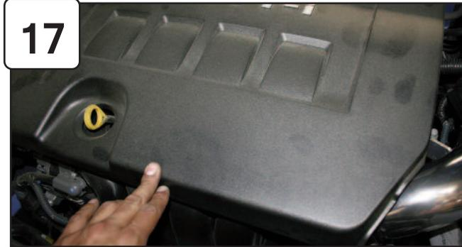
Re-install engine cover. Re-connect battery terminals.
