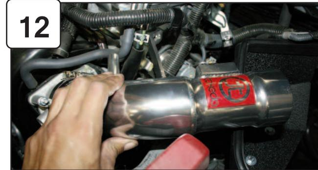
Install intake assembly and position. Do not tighten.
