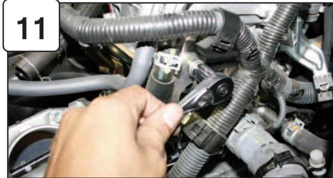
Loosen bolt on side of engine using 13mm socket or wrench.
