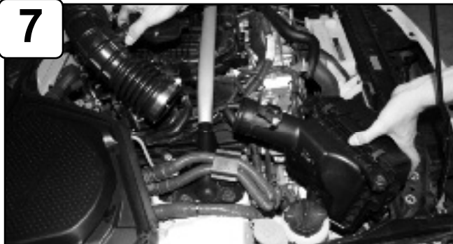
Remove complete intake out of vehicle.
