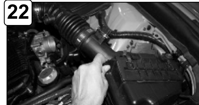
Remove complete intake out of vehicle.
