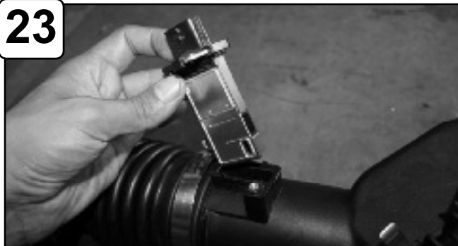
Remove MAF sensor from stock intake.
