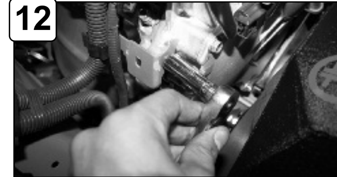
12 Loosen bolt on engine securing harness bracket.
