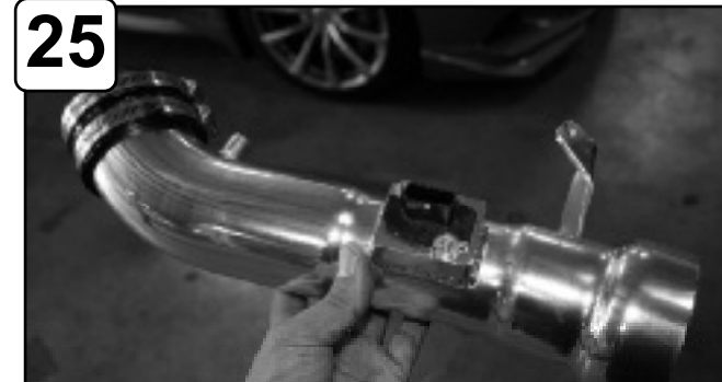
Attach coupling with clamps to tube.
