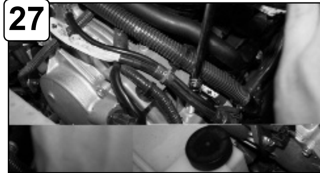
Loosen bolt on engine securing harness bracket.
