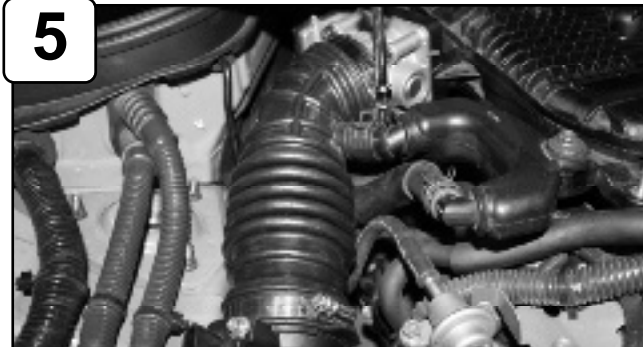
Loosen clamps on intake using 5/16" nut driver.
