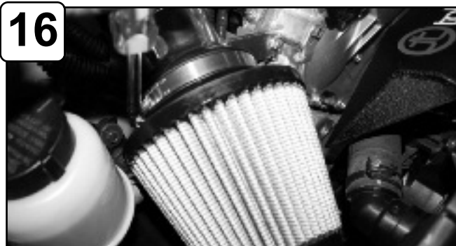
16 Install air filter and tighten using 5/16" nut driver.
