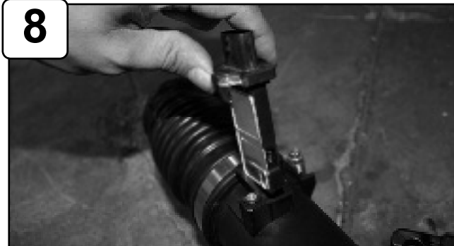
Remove MAF sensor from stock intake.
