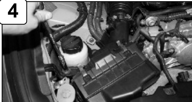
Disconnect MAF sensor harness. With 10mm socket or wrench loosen bolt holding in air box.
