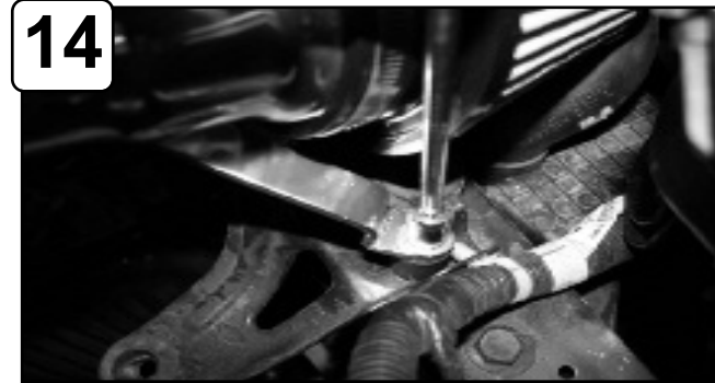
14 Using provided flat washer and nut, secure tab using 13mm socket or wrench.
