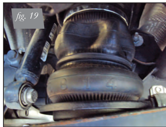
Installation with factory shock, roll plate and un-cut lower bracket
