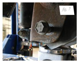
4. Reinstall the stabilizer bar (figs. 8 and 9). Torque bolts to 47 Nm (35 ft-lbs.).
