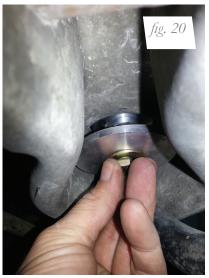
Remove the shock rod nut, upper washer and bushing from the new shock. Insert the shock into the shock tower, aligning the lower mount hole with the shock mounting bracket and insert the lower shock bolt through the mount (figs. 21-23). Do not torque at this time.
