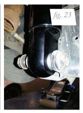
7. Apply the upper bushing, washer and shock rod nut (fig. 24). Torque the rod nut to 27 Nm (20 ft-lbs.) (fig. 25). Thread the damping adjuster onto the rod (fig. 26).
