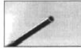
Good cut - clean and square
