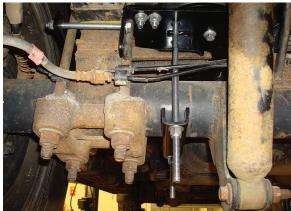
Image shows the right (driver side) rear view of the lower bracket and hardware in position.
