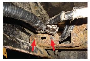
Remove the line holders from the gas/urea tank bracket for easier access to the upper brace hardware.
