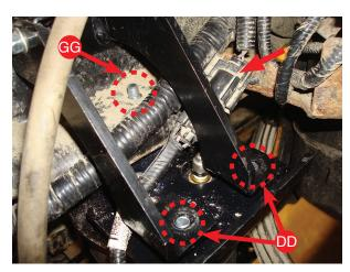
Raise the axle up while aligning the 3/8"-16 x 2.00" carriage bolt through the frame and the two 3/8"-16 X 1.25" carriage bolts in the upper bracket, through the brace.
