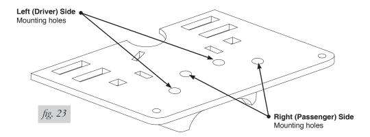
This slot should be on the opposite side of the fitting on the bellows once mounted.
