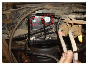
Tighten the 8mm hardware and the 1/2" (or 3/4" if from the 5th wheel hitch hardware) and tighten securely. Repeat for the hardware on the opposite side.
