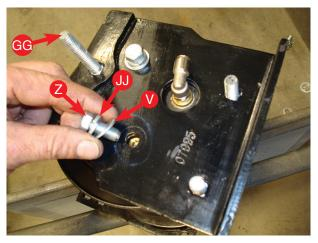
Attach the upper bracket to the bellows assembly with two 3/8" flat washers (V), 3/8" lock washers (JJ), and 3/8"-24 x 7/8" hex head cap screws (Z).
