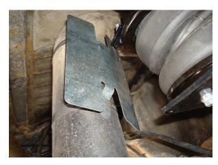
The shield is shown in position with air gap between it and the exhaust pipe.
