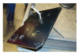
For the passenger side lower bracket, insert the 3/8"-16 x 10" carriage bolt (EE) through the square hole as shown in the picture and in figure 20.
