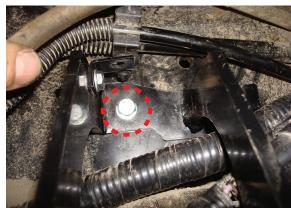
Attach the bracket to the frame using the M8 hardware noted.
