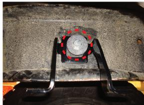
Passenger side upper brace shown with hardware supplied in place.
