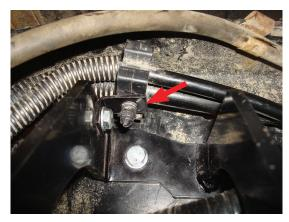
Insert the line holder previously removed into the L-bracket installed on the upper brace as shown.
