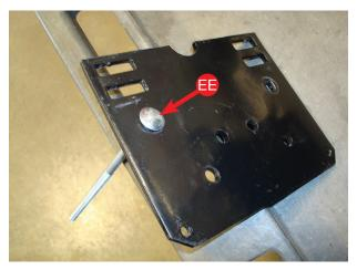
For the driver side lower bracket, insert the 3/8"-16 x 10" carriage bolt (EE) through the square hole as shown in the picture and in figure 20.
