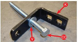
Insert the 3/8"-16 x 5" hex tap bolt and 3/8" flat washer through the top round hole of the four hole locating bracket (closest to the bend) first.
