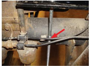
Make sure when setting the left side in place (driver side) that the 3/8"-16 x 10" carriage bolt goes in between the axle and the hard brake/ ABS line.
