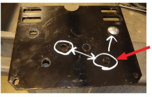
bellows mounting holes shown in location to the 3/8"-16 x 10" carriage bolt previously installed. When installing on the bellows, make sure the bracket edge facing you is on the fitting side of the bellows.
