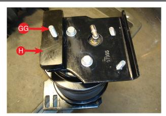
Spacer (H) set on bracket and in position. The wide portion will face the outside of the vehicle.
