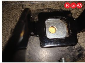
For the passenger side, before inserting the upper brace hardware, make sure that the 1/2" thick washer (R) or (AA) is installed in between the brace and frame (see Step 2).
