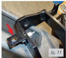
No matter what side the L-bracket is on, make sure it is installed so the flat side points up when tightening.
