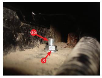
Install the 3/8" -16 serrated flange lock nut (S) onto the 3/8"-16 x 2.00" carriage bolt that goes through the flange on the frame and tighten securely.
