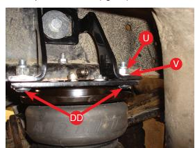
Cap the 3/8"-16 x 1.25 carriage bolts with 3/8" flat washer and 3/8" Nyloc nut and torque to 15ftlbs. Repeat for both sides.
