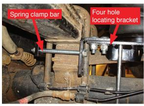
With the spring clamp bar tight so that the lower bracket is up against the stock U-bolts, the four hole locating bracket should be forward and behind the U-bolts as shown. Note the lower bracket being parallel with the leaf spring.
