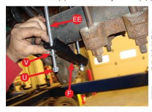
Set the axle clamp bar over the 3/8"-16 x 10" carriage bolts and cap with 3/8" flat washer and 3/8" Nyloc nut. Leave loose at this time.
