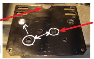
Driver side bellows mounting holes shown in location to the 3/8"-16 x 10" carriage bolt previously installed. When installing on the bellows, make sure the bracket edge facing you is on the fitting side of the bellows.
