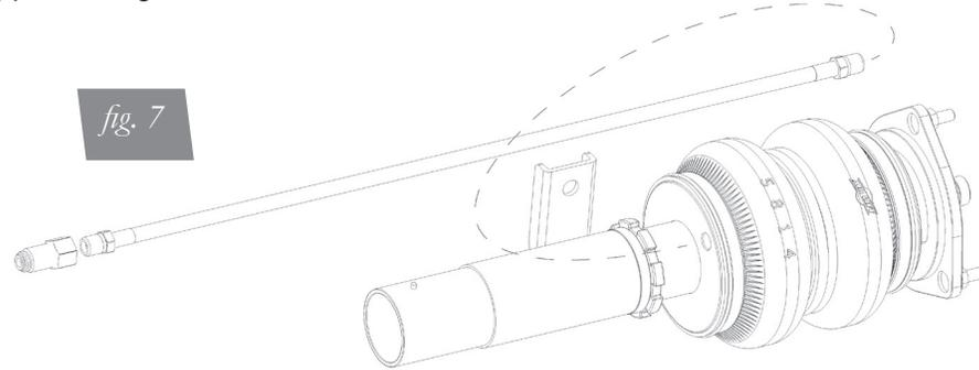
2. Insert strut into the hub assembly. Reinstall the lower mounting bolt and torque to 70 Nm (52 lb-ft).
