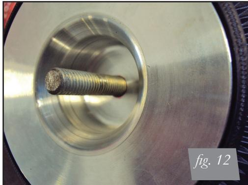
9. Wrap the threads of the fitting with Teflon tape or thread sealant. Tighten the fitting 1 3/4 turns beyond hand tight.
