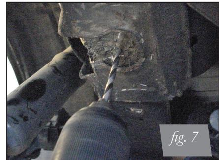
7. Assemble the nutsert and nutsert tool together and insert into the 17/32" hole. Review diagram below on how to attach the nutsert to the vehicle. (fig. 8).
