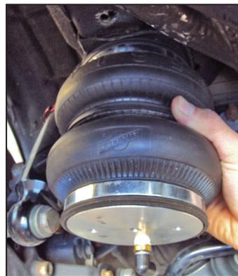
11. Orient the air fitting inline with lower transverse link toward the center of the vehicle.
