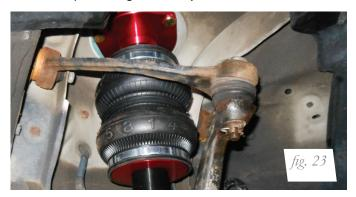
5. Reassemble the stabilizer bar to the stabilizer bar end link (fig. 24). Torque both the nut and bolt to 55Nm (43lb-ft).
