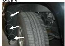
Remove the three torx screws from the side of the wheel well
