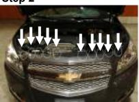
Remove the ten torx screws located on the top of the grille
