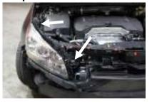
Remove the two 7mm bolts from the top of the headlight housing
