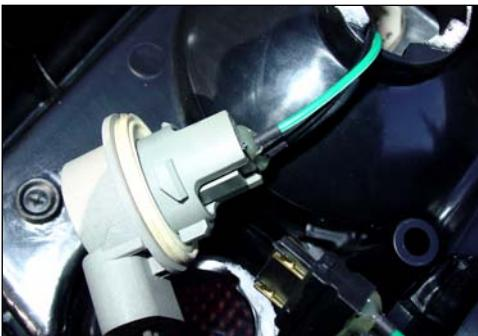
Plug the pigtails into the stock harness making sure the wires line up black to black. Be sure to secure the reverse bulb in tact.
