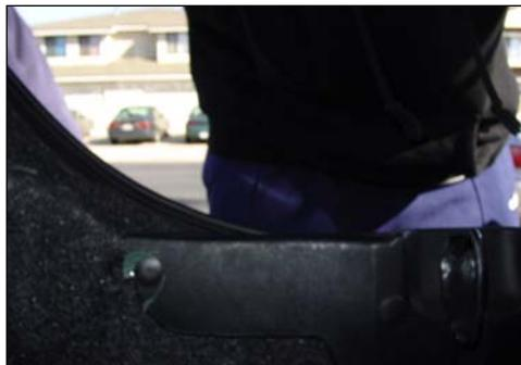
Remove the four pins to remove the plastic cover.
