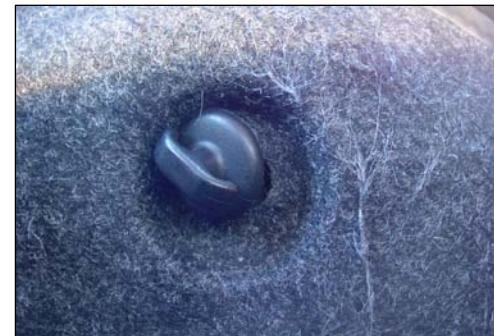
Remove the plastic screws to remove the carpet cover.
