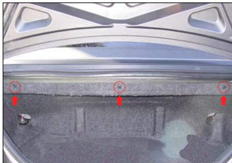
Remove the three plastic push pins that hold the top carpet shroud.
