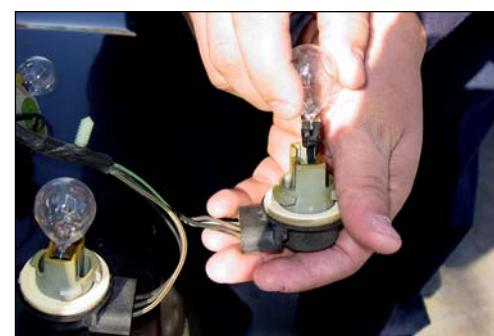
Remove the bulbs from the socket leaving the reverse bulb intact for you will need it for the new L.E.D taillights.
