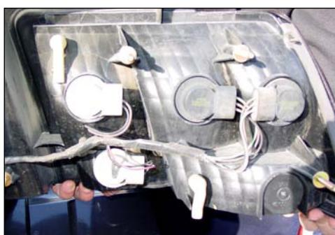
Pull the taillight housing straight out, twist and pull the plugs as if you were changing the bulbs.
