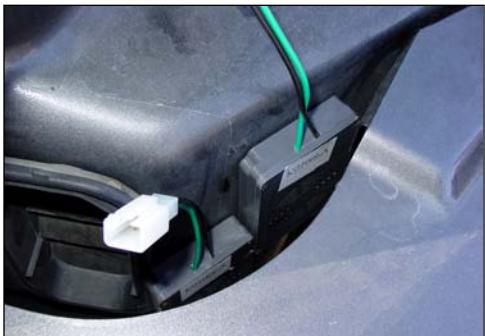
Place the resistor boxes behind the bumper and out of the way of the taillight housing.
