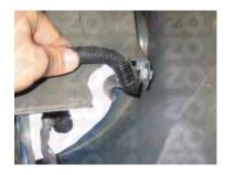
Step 3: Unclip the wire harness from the frame.
