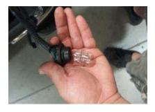
Once you have removed the sockets from the housing. Remove the bulbs from the sockets. Leave the reverse bulb alone.
