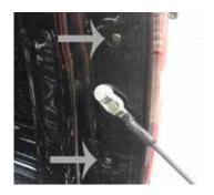
Remove the 2 Torx screw holding the taillight in.
