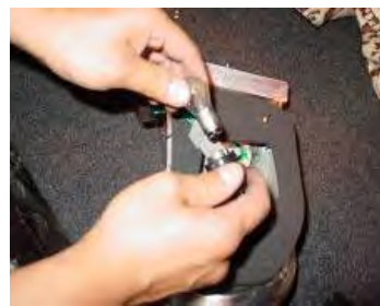
Step 10: Remove the bulb from the black socket also remove the 194 bulb this will not be used.
