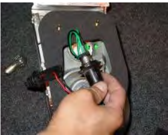
Step 11: Plug in the adaptor from the new tail light into the black socket.
