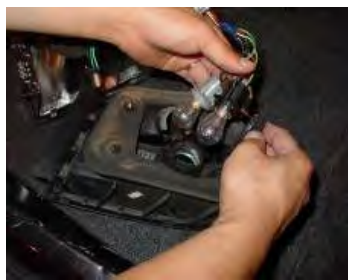
Step 9: Twist off the bulb wire harness from the original tail light.
