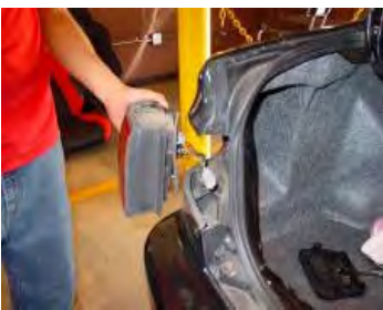
Step 8: Unplug the wire harness and remove the tail light.
