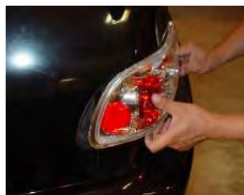
Step 12: Put on the new Anzo tail light and screw it on.
