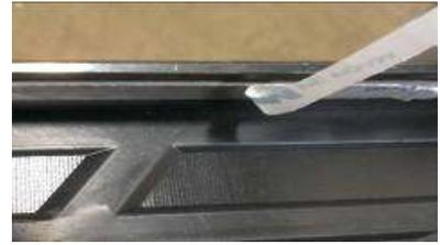
Now that the wires are ran through the tailgate you can peel off the paper strip across the back of the tailgate bar. This 3m tape is to secure the back of the spoiler like factory.
