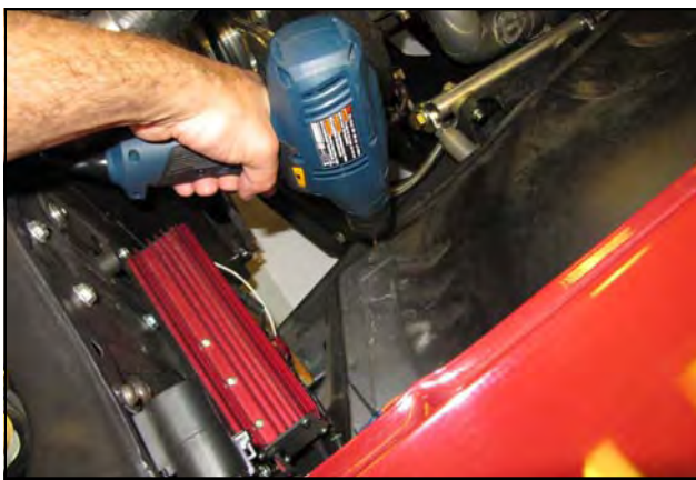
10. Drill 1/8" pilot holes into the inner fender.
