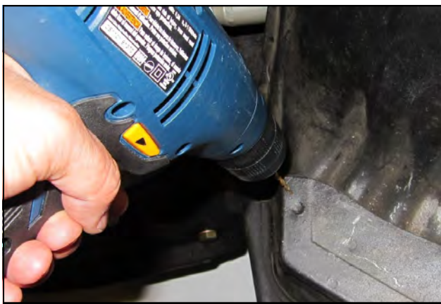
10. Drill 1/8" pilot holes into the inner fender.
