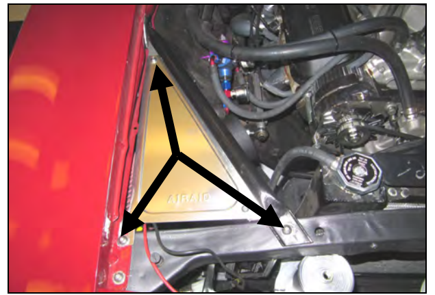
12. Install the assembly into the inner fender. Reinstall the fender support on top of the Airaid brackets and secure using the factory hardware. Reinstall the fender bolt removed in step 7.
