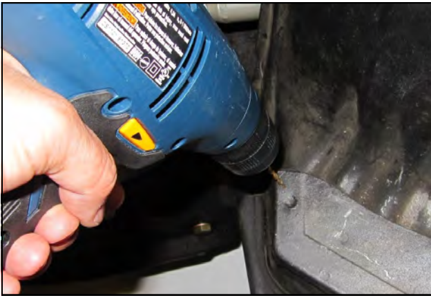
10. Drill 1/8" pilot holes into the inner fender.
