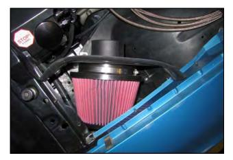
**10.** Install the Airaid premium onto the Filter adapter and tighten the clamp..
