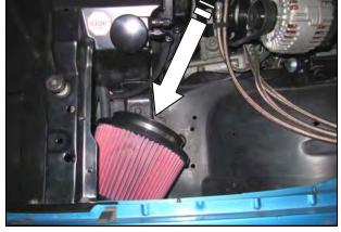
**5.** Tuck the Airaid premium Filter (#1) into the inner fender.
