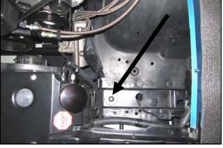
**3. Driver Side** - Remove the inner fender bolt and set it aside. It will be re used in step #7.
