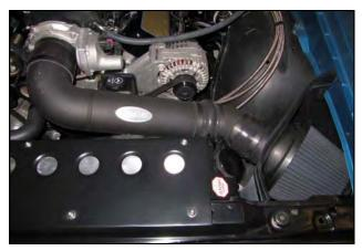
14. Connect the performance airbox assembly to your throttle body or carburetor by using any combination of Airaid's UBI components.
