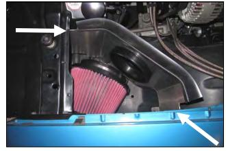
**6.** Carefully install Air Dam assembly in to the inner fender area. **Note-**The outermost edges will be underneath the core support and the fender when installed properly.
