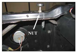
**4.** Install the L bracket (#5) under the core support .Use the 5/16 Flange nut (#7) to secure it to the lower portion of the hood stop.
