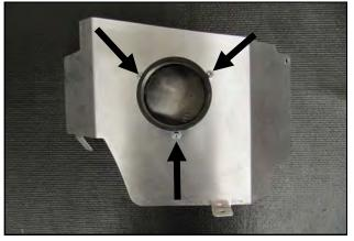
1. Remove the protective film from the sheet metal. Install the Filter Adapter (#3) onto the Air Dam (#2) using three sets of 1/4-20 Button Head Bolts (#7), and 1/4" Flat Washers (#8).
