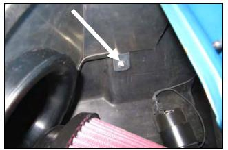
**9.** The third mounting point will need to be drilled into the inner fender. Secure the Air Dam tab using one 1/4-20 Button Head Bolt, one 1/4" Flat Washer topside, and the Fender Washer (#10) and the last 1/4-20 Nylock nut from below.
