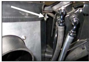
**8.** Attach the L bracket to the Air Dam using one 1/4-20 Button Head Bolt, Two 1/4" Flat Washers, and one of the 1/4-20 Nylock Nuts (#11).
