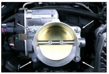
**4.** With a 10mm socket remove the two nuts, and the two bolts that hold the throttle body to the intake manifold. Without disconnecting the wiring harness, set the throttle body aside.
