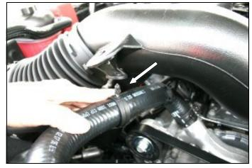
**Disconnect the negative battery cable!** 1. Lift up on the front of the and beauty cover and remove it from the vehicle. Push down on the radiator hose, and separate the intake tube from the plastic clamp.
