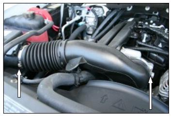
**3.** Next loosen the hose clamp on the intake tube at the throttle body, and at the Mass Air Sensor, and then remove the tube from the vehicle.
