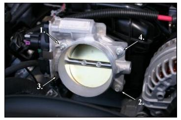
**6.** Reinstall the throttlebody onto the intake manifold using the factory hardware. Tighten the nuts and bolts in a cross pattern to the vehicle manufacturer's specifications. Before starting the engine, open and close the throttlebody to make sure there are no obstructions.
