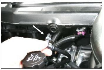
2. Disconnect the breather tube from the intake tube, by gently pulling towards you. An O-ring is all that holds it in place.
