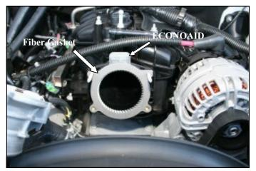
**5.** Install the ECONOAID Throttlebody Booster against the manifold over the studs with the logo facing the throttlebody. Next install the supplied gasket against the ECONOAID.
