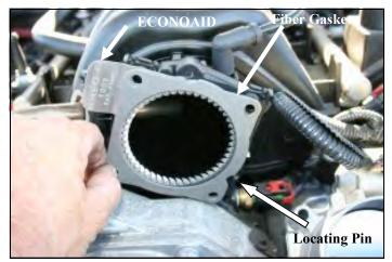
3. Install the ECONOAID Throttlebody Booster against the intake manifold with the logo facing the front of the vehicle and the supplied gasket on the throttlebody side of the plate. Make sure to align the two locating pins correctly with the notches in the ECONOAID and the gasket.
