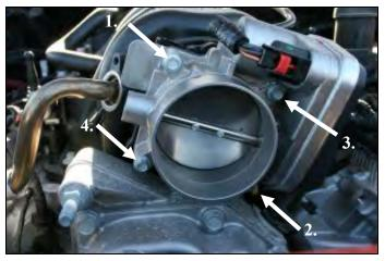
4. Reinstall the throttlebody using the factory bolts. Tighten them using a cross pattern to the manufacturer's specifications. Before starting the engine, open and close the throttlebody to make sure there are no obstructions.
