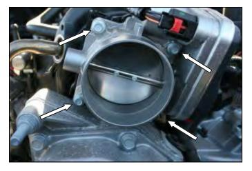
**2.** Using a 5/16" socket, remove the four bolts that hold the throttlebody to the intake manifold.
