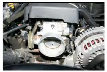
**5.** Now reinstall the three studs, and nuts and tighten them to the manufacturer's specifications. Before starting the engine, open and close the throttlebody to make sure there are no obstructions.
