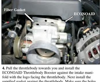
**4.** Pull the throttlebody towards you and install the ECONOAID Throttlebody Booster against the intake manifold with the logo facing the throttlebody. Next install the supplied gasket against the throttlebody. Make sure the holes in the gasket align with the holes in the ECONOAID. (If your vehicle does not have an O-ring in the face of the intake manifold, install the second supplied gasket between the ECONOAID and the manifold).
