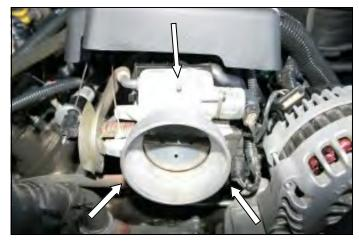
**3.** Using a 4mm socket, remove the three studs that go thru the throttlebody into the intake manifold
