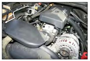
Disconnect the negative battery cable! Loosen two hose clamps and remove the air intake tube. Separate the intake tube from the plastic clamp on the upper radiator hose. (If equipped).
