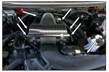
**5.** Reinstall the intake tube and tighten the five bolts. Reconnect the mass air sensor. Reconnect the crankcase breather hose.
