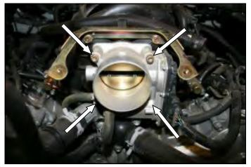
**3.** Remove the four bolts that hold the throttlebody to the intake manifold.
