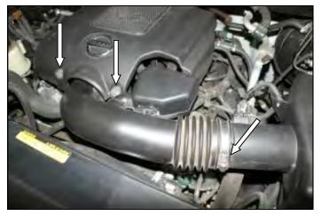
**6.** Reinstall air intake tube between the throttlebody and the airbox and tighten the clamps. Reinstall the beauty cover and tighten the bolts.
