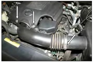
1. **Disconnect the negative battery cable!** Remove the two bolts that secure the engine beauty cover, and then remove it from the vehicle. Loosen the hose clamp that secures the air intake tube to the airbox.
