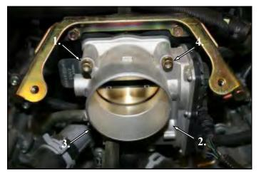
**5.** Reinstall the factory bolts and tighten the bolts in a cross pattern to the manufacturer's specifications. Before starting the engine, open and close the throttlebody to make sure there are no obstructions.
