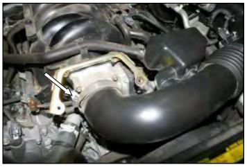
**2.** Loosen the hose clamp that secures the air intake tube to the throttlebody and then remove the tube from the vehicle.
