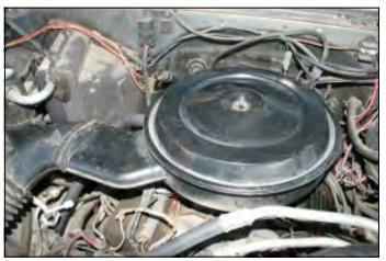
**5.** Reinstall the air cleaner and reconnect the crankcase breather hose, and the plastic fresh air tube.
