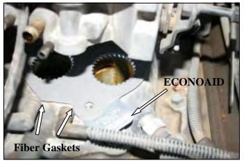
**3.** Carefully lift the throttlebody straight up and slide the ECONOAID Throttlebody Booster with one gasket on each side and the logo facing up, into position on top of the intake manifold. Make sure that the bolt holes in the ECONOAID and the two gaskets are aligned over the bolt holes in the intake manifold, and then reinstall the throttlebody.
