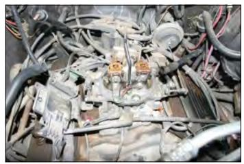
**2.** Disconnect the three vacuum lines on the front of the throttle body, and disconnect the throttle cable and cruise control cables. Next remove the three bolts that secure the throttle body to the intake manifold.
