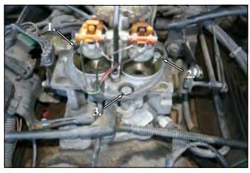
**4.** Reinstall the factory bolts thru the throttlebody and tighten them to the manufacturer's specifications. Reconnect the vacuum hoses and throttle cables. Before starting the engine, open and close the throttlebody to make sure that there are no obstructions.
