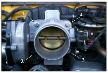
**4.** Reinstall the throttlebody onto the intake manifold using the factory hardware. Tighten the nuts and bolts in a cross pattern to the vehicle manufacturer's specifications. Before starting the engine, open and close the throttlebody to make sure there are no obstructions.
