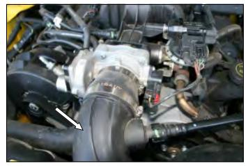
1. <u>Disconnect the negative battery cable!</u> Remove the air intake tube between the air filter housing and the throttlebody.
