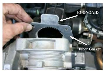
**3.** Install the ECONOAID Throttlebody Booster and supplied gasket between the throttlebody and the intake manifold with the logo facing the front of the vehicle. Make sure that the gasket is between the throttlebody and the ECONOAID. (*If your application does not have an O-ring on the intake manifold, install the second supplied gasket between the ECONOAID and the intake manifold*).
