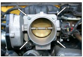
**2.** Remove the four bolts that hold the throttlebody onto the intake manifold.
