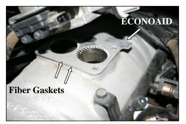
**5.** Install the ECONOAID Plate against the manifold with one gasket on top of the plate, and one gasket under the plate with the ECONOAID logo facing the throttlebody.
