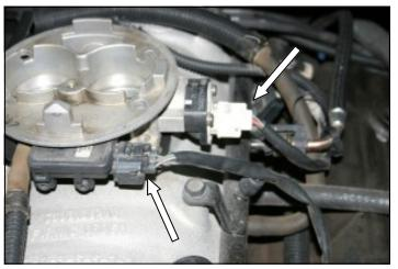
**4.** Disconnect the two electrical connectors on the drivers side of the throttle body.
