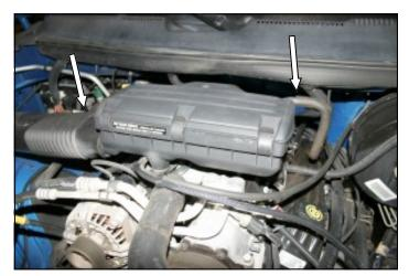
1. <u>Disconnect the negative battery cable!</u> Disconnect the crankcase breather hose, and the fresh air intake tube from the air filter housing.
