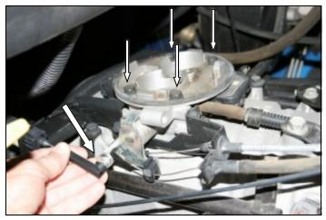
**3.** Push the transmission cable end towards the front of the vehicle to unhook it from the linkage arm. Next remove the four bolts that secure the throttlebody to the intake manifold.
