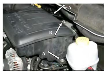
**2.** A.) Using a 10mm socket, remove the two bolts that secure the resonator to the engine. B.) Using a 5/16" socket, loosen the hose clamp that secures the rubber coupler on the back of the resonator to the throttlebody. Lift the front of the resonator straight up to disengage it from the mounting grommet, and remove the resonator assembly from the vehicle.
