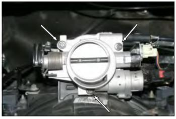
**3.** Remove the 3 bolts that secure the throttlebody to the intake manifold.
