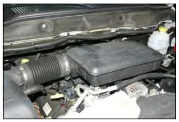
**6.** Reinstall the resonator and intake tube in the reverse order that they were removed. Make sure to reconnect the air temperature sensor.
