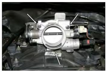
**5.** Reinstall the throttlebody onto the intake manifold and tighten all three bolts to the vehicle manufacturer's specifications. **Before starting the engine**, open and close the throttlebody to make sure there are no obstructions.
