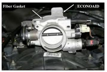
**4.** Install the supplied gasket between the ECONOAID Throttlebody Booster and the throttlebody making sure that the logo on the ECONOAID is facing the throttlebody.
