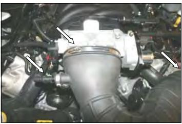
**5.** Reinstall the intake tube and tighten the two hose clamps. Reconnect the crankcase breather tube onto the intake tube.
