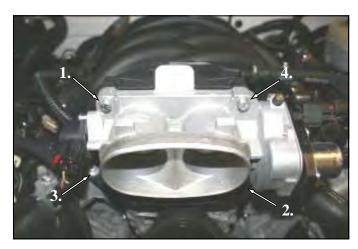
**4.** Reinstall the throttlebody onto the intake manifold using the factory hardware. Tighten the bolts in a cross pattern to the vehicle manufacturer's specifications. Before starting the engine, open and close the throttlebody to make sure there are no obstructions.
