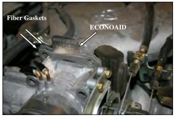
**3.** Install the ECONOAID Throttlebody Booster against the intake manifold with the logo facing the throttlebody. Next install the supplied gaskets, one on each side of the ECONOAID.
