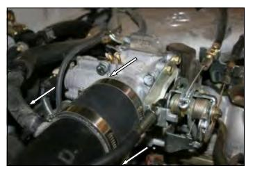
**5.** Reinstall the intake tube and tighten the hose clamps. Reconnect the crankcase breather hose.
