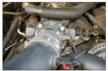
**5.** Reinstall the intake tube and tighten the hose clamps. Reconnect the air intake temperature sensor. Reconnect the crankcase breather hose.
