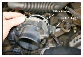
**3.** Install the ECONOAID Throttlebody Booster against the intake manifold with the logo facing the throttlebody. Next install the supplied gasket between the ECONOAID and the throttlebody.
