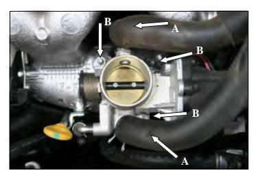
**2.** A.) Disconnect the two rubber hoses from the throttlebody. B.) Remove the two nuts and one bolt that secure the throttlebody to the intake manifold.
