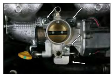
**4.** Reinstall the throttlebody onto the intake manifold and tighten the two nuts and one bolt to the vehicle manufacturer's specifications. Before starting the engine, open and close the throttlebody to make sure there are no obstructions. Reconnect the two rubber hoses to the throttlebody.
