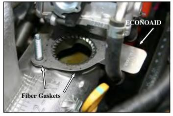
**3.** Lift the throttlebody off of the intake manifold and remove the old gasket. Install one supplied gasket against the intake manifold, and then the ECONOAID Throttlebody booster with the logo facing the throttlebody. Next install the remaining gasket between the ECONOAID and the throttlebody.
