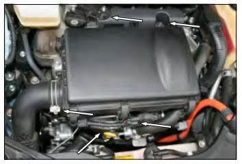
**5.** Reinstall the air cleaner box onto the top of the throttlebody. Reconnect the fresh air tube and tighten the clamp. Tighten the clamp on the throttlebody. Reinstall the two bolts that secure the airbox to the engine. Reconnect the Mass Air sensor wiring harness.
