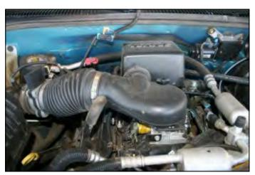
**5.** Reinstall the intake hat and tighten the wing nut. Reconnect the crankcase breather hose. Reconnect the intake tube and tighten the clamp.
