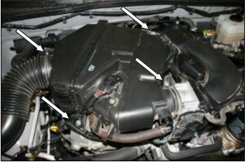
**2.** Loosen two hose clamps, one at the fresh air tube, and one at the throttlebody. Remove two bolts that secure the airbox to the engine.
