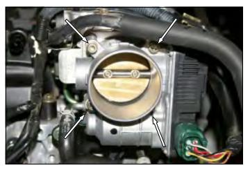
**5.** Reinstall the throttlebody onto the intake manifold and tighten all four bolts to the vehicle manufacturer's specifications. Before starting the engine, open and close the throttlebody to make sure there are no obstructions. Reinstall the intake tube and the beauty cover in the reverse order that they were removed.
