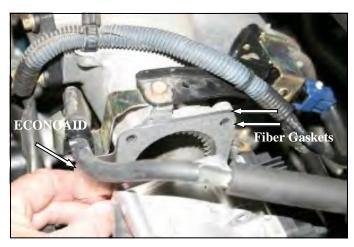
**4.** Install one of the supplied gaskets on each side of the ECONOAID Throttlebody Booster and then install the ECONOAID between the intake manifold and the throttlebody making sure that the logo is facing the throttlebody.
