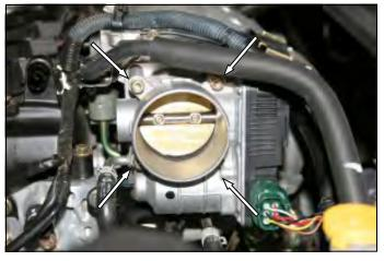
**3.** Remove the 4 bolts that secure the throttlebody to the intake manifold. Remove the throttlebody from the intake manifold and remove the old gasket.
