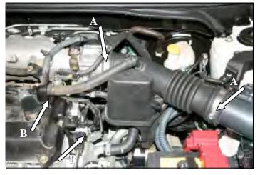
**2.** A.) Loosen the two hose clamps that secure the air intake tube between the air cleaner box and the throttlebody. B.) Using pliers, squeeze the hose clamp that secures the crankcase breather hose to the valve cover and slide the it up the breather hose so it won't get lost. Remove the intake tube assembly and set it aside.
