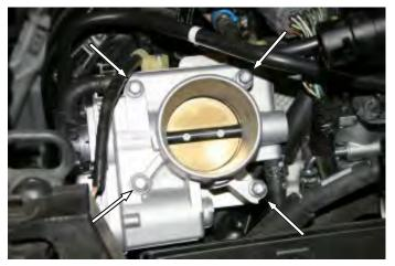
**5.** Make sure all of the holes are aligned, and then reinstall the factory bolts and tighten them to the factory specifications. Before starting the engine, open and close the throttlebody to make sure there are no obstructions. Reinstall the intake tube, air cleaner lid, fresh air duct, battery cover, and the beauty cover in the reverse order that they were removed.
