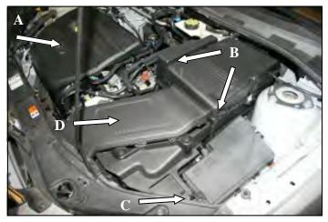
A.) Carefully lift straight up on the engine beauty cover and remove it from the engine. (*It is only held on by grommets.*)
