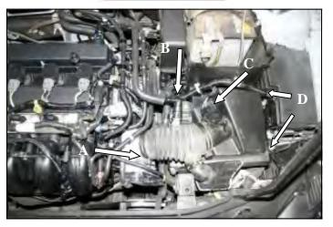
**2.** A.) Loosen the hose clamp that secures the air intake tube to the throttlebody. B.) Disconnect the crankcase breather from the air intake tube. C.) Disconnect the mass air sensor wiring connector from the mass air sensor on the air intake tube. D.) Unlatch the four clips (*one on each corner*) that secure the air cleaner lid to the lower airbox. Remove the air cleaner lid and flexible air intake tube from the vehicle as an assembly. Now remove the air cleaner from the lower airbox.
