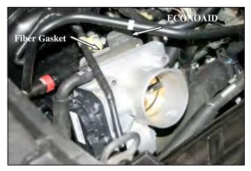
**4.** Pull the throttlebody away from the intake manifold. Install the ECONOAID Throttle Booster (*with the logo facing the throttlebody*) and the supplied gasket between the throttlebody and the intake manifold. The gasket needs to be between the intake manifold and the ECONOAID.
