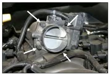
**4.** Reinstall the factory bolts thru the throttlebody and ECONOAID Booster and tighten to the manufacturer's specifications.
