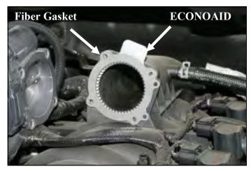
**3.** Install the ECONOAID Booster onto the intake manifold as shown. (*The tab on the ECONOAID Booster may be rotated 90° to the left if desired.*) Now install the gasket and make sure it is seated correctly over the two alignment pins on the intake manifold. Make sure the ECONOAID logo faces the throttlebody.
