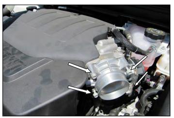
**3.** Remove the four bolts that secure the throttlebody to the intake manifold. It may also be necessary to remove a wiring bracket depending on your application.
