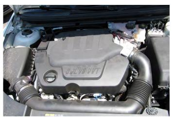
**5.** Reinstall the intake tube, and any other parts that were removed to gain access to the throttlebody in the reverse order in which they were removed.
