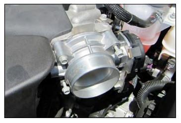
**4.** Pull the throttlebody away from the intake manifold and Install the ECONOAID Throttle Booster and supplied gaskets. The logo is to be facing the throttlebody and in the 12:00 o'clock position. the supplied gaskets, are to be on either side of the ECONOAID.
