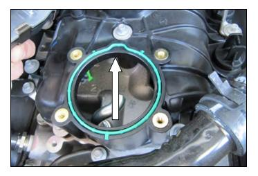
**5.** Chevrolet Silverados and GMC Sierras have composite manifolds and use an O-ring type gasket. If your vehicle has an O-ring type gasket, place the Econoaid directly on top of the O-ring, and one fiber gasket on top of the Econoaid. Do not use the second fiber gasket.
