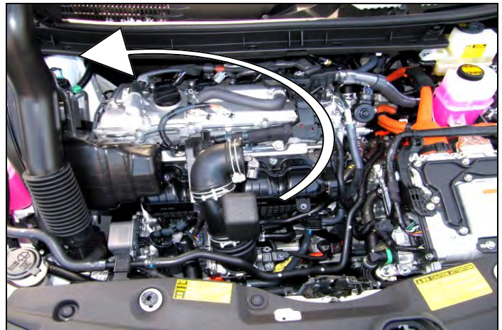
6. Rotate the factory airbox and tube assembly to the passenger side of the engine compartment and stand it up vertically.
