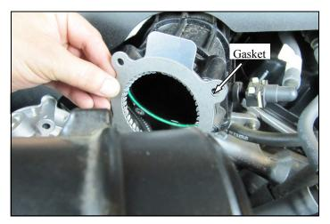
**3.** Pull the throttle body away from the intake manifold and Install the ECONOAID Throttle Booster and the supplied gasket. The logo is to be facing the throttle body and in the 12:00 o'clock position. the supplied gasket is to be on throttle body side. Align the bolt holes, and reinstall the factory bolts. Tighten the bolts to the factory specifications in an "X" pattern. Before starting the engine, manually cycle the throttle plate to make sure there are no obstructions.
