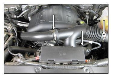
1. Locate and loosen the intake tube clamps. Remove the factory intake tube and set it aside. It may be necessary to remove the engine cover to gain access to the throttlebody on some applications.
