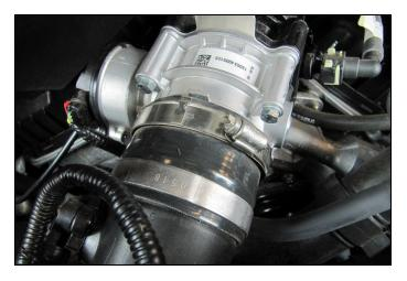
**4.** Slide the throttle body inlet tube back onto the throttle body and tighten the clamp.
