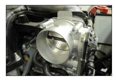
**5.** Align the bolt holes, and reinstall the factory bolts. Tighten the bolts to the factory specifications in an "X" pattern. Before starting the engine, manually cycle the throttle plate to make sure there are no obstructions.
