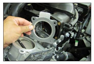
**4.** Pull the throttlebody away from the intake manifold and Install the ECONOAID Throttle Booster and supplied gasket. The logo is to be facing the throttlebody and in the 12:00 o'clock position. the supplied gasket, is to be on the throttlebody side of the ECONOAID.
