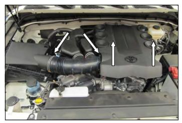
1. Locate and loosen the intake tube clamps on both the throttlebody and the airbox. Remove the factory intake tube and set it aside. It may be necessary to remove the engine cover to gain access to the throttlebody on some applications.
