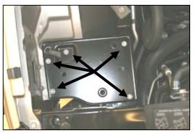
**5.** Remove 5 bolts, and remove the factory airbox mounting plate.
