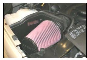
**11.** Install the Airaid Premium Filter (#1) onto the filter adapter (#4), and tighten the hose clamp. Next install the weather strip (#5) onto the top of the CAD as shown. For ease of installation start at the fender, and work towards the radiator.
