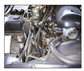
**4.** Rock the factory air box back and forth and remove it from the vehicle. There are only grommets holding it in, no bolts.
