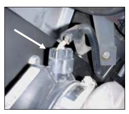
11. Reconnect the wiring harness to the MAF sensor.
