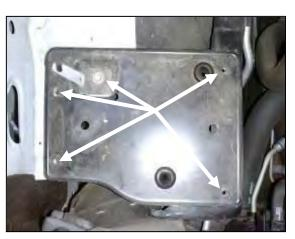
5. Using a 10mm socket, remove the five bolts that secure the factory air filter housing platform and
