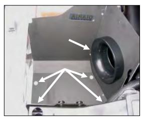
7. Install the air filter adapter (#4) using three  $\frac{1}{4}$ -  $20x \frac{1}{2}$ " button head bolts (#12), and 1/4" flat washers (#13). Position the Airaid Cool Air Dam in place of the factory airbox & secure it with four M6-1x25 hex bolts (#14) and 1/4" flat washers (#13).
