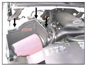
**12.** Press the weather strip (#8) along the top edges of the Airaid Cool Air Dam; assure that it is fully seated along the edges. (Hint: *Begin at a corner and work toward the ends*). Mount the Airaid Premium Filter (#1) onto the air filter adapter and tighten the hose clamp.
