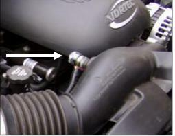
1. <u>Disconnect negative battery cable.</u> Remove the factory filter minder and rubber grommet from the factory intake tube, retain for re-installation later in the install.
