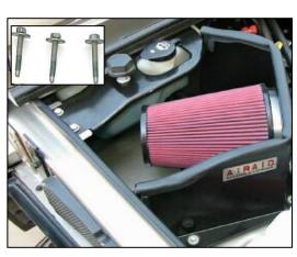
**9.** Position the Airaid system over the three factory mounting points & secure with the three saved factory bolts removed in step #4.
