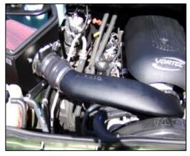
**13.** Connect the Airaid MIT (#5), hump hose end first, to the MAF sensor, and then connect the other end of the tube assembly to the throttle body. Check for interference and adjust the MIT accordingly, then tighten the hose clamps.
