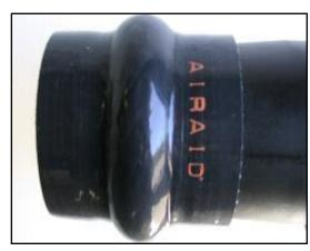
**12.** Install the provided silicone hump hose (#7) onto the Airaid Modular Intake Tube (MIT) (#5) with the 2 supplied #56 hose clamps (#12). **Note:** Leave hose clamps loose until final assembly.
