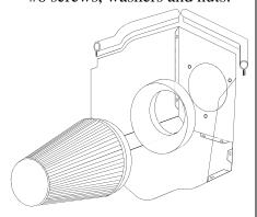
6. Using the three supplied \( \frac{1}{4} - \) 20 bolts and washers, install the air filter adaptor on the Airaid Cool Air Dam.
