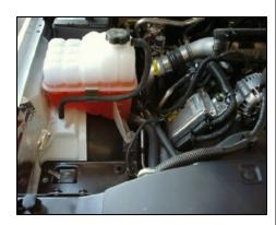
**3.** Loosen hose clamps on factory intake tube assembly and remove from engine. Unsnap factory air box assembly and remove from vehicle.
