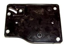
**4.** Using a 10mm socket, remove the five bolts and plate from engine compartment.
