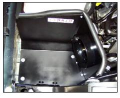
7. Install Airaid Cool Air Dam assembly in engine compartment using the supplied bolts and washers.
