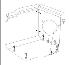
**5.** Assemble Airaid Cool Air Dam panels using the supplied #6 screws, washers and nuts.
