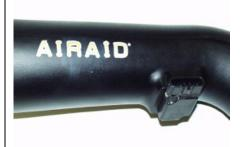
**8.** Using the supplied 8/32 allen head bolts and washers, install factory mass air sensor in Airaid intake tube. (Note: Sensor must be installed in direction shown in picture.)
