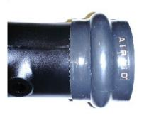
10. Install supplied hump hose and two #64 hose clamps onto large end of Airaid intake tube. (Note: Leave hose clamps loose until final assembly.)
