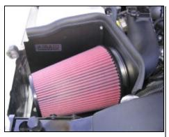
13. Install the supplied Airaid filter on the air filter adaptor. Install the supplied weather strip on the Airaid Cool Air Dam. (Note: Start from one corner and work your way around to insure proper alignment of weather strip.)
