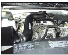
12. Install Airaid intake assembly onto engine. Position coupler and hump hose and tighten hose clamps. (*Note: There should be a gap in between the Airaid intake tube and the air filter adaptor.*)
