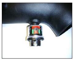
**9.** Install factory rubber grommet and air filter minder in Airaid intake tube.
