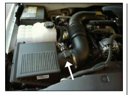
1. Disconnect **negative** battery cable. Using supplied T-20 security bit, remove factory mass air sensor (save for later use).
