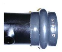
**10.** Install supplied hump hose and two #64 hose clamps onto large end of Airaid intake tube. (<u>Note</u>: Leave hose clamps loose until final assembly.)
