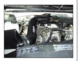
**12.** Install Airaid tube assembly onto engine. Position coupler and hump hose and tighten hose clamps. Connect wire harness to mass air sensor. (<u>Note</u>: There should be a gap between the Airaid intake tube and the air filter adaptor.)
