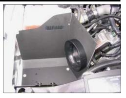
7. Install Airaid Cool Air Dam assembly in engine compartment using the four supplied bolts, and washers.
