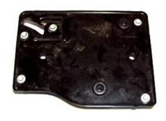
**4.** Using a 10mm socket, remove the five bolts and plate from engine compartment.
